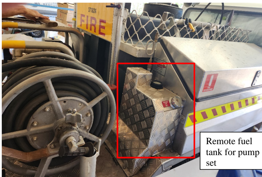
Figure 1 - Remote fuel tank (being removed) shown above with pump set and hosereel to its left.
