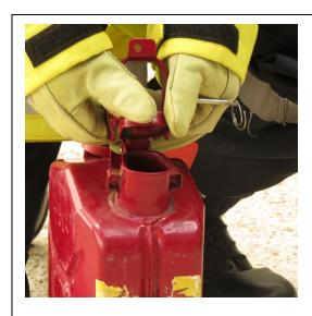
6. Allow for full pressure venting under control before fully opening
