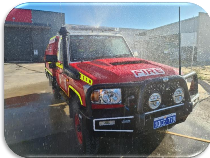
Figure 4.30 - Deluge System in Operation
