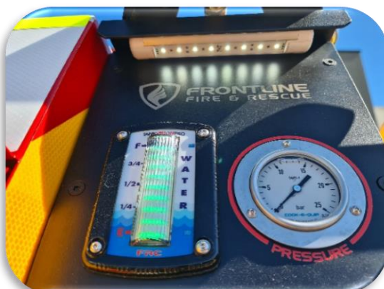
Figure 4.54 - Pump Panel Lighting
