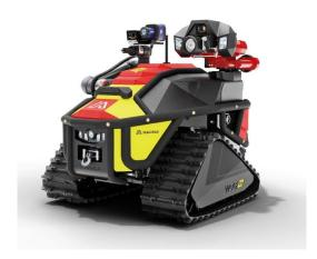
The primary capability of the Magirus Wolf R1 is as a remotely controlled water monitor delivering 2000l/min at 10 bar with a throw distance of 65 metres for water and 45 metres for foam.
